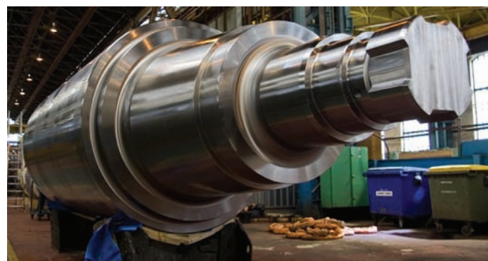
One of Sheffield Forgemasters' large back-up rolls.
