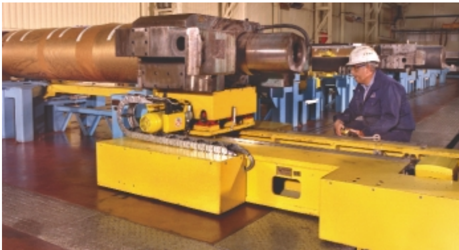
Work roll chock strip and build equipment designed by Parkegate Engineering
