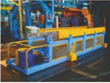
Parkegate designed this rapid work roll change rig
